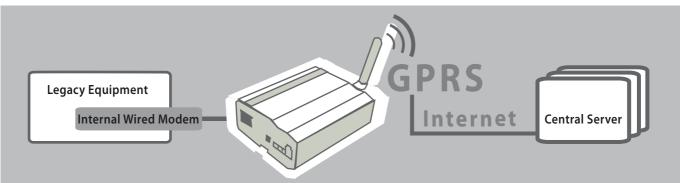
The BridgeD130 is the easiest way to switch legacy equipment from traditional phone landlines to the wireless GSM/GPRS network. The phone network cable is connected directly to the BridgeD130 that extracts the payload data from the modem flow.
